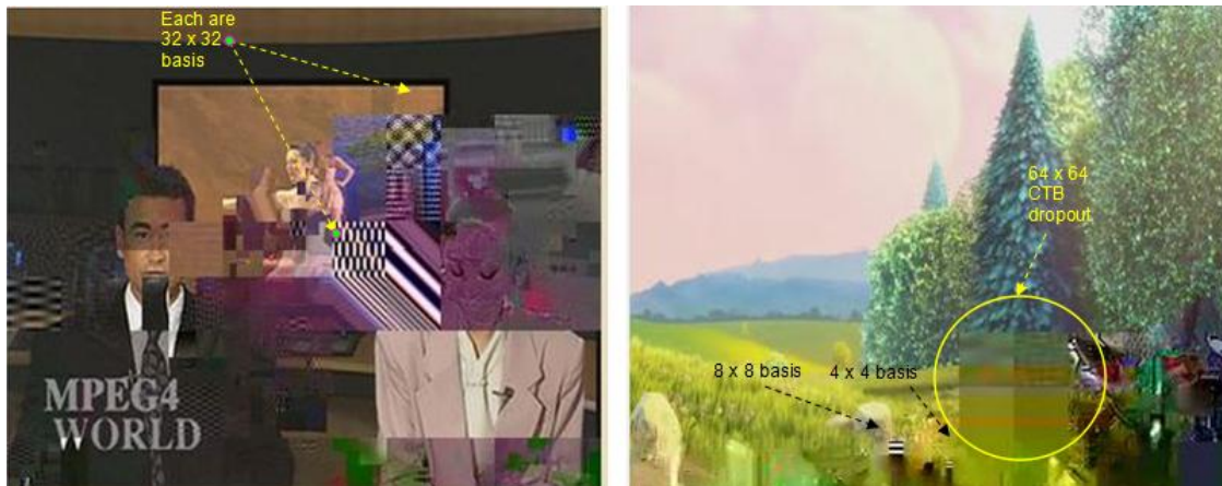
Examples of how HEVC video failure / dropout profiles will consequently affect 4K
